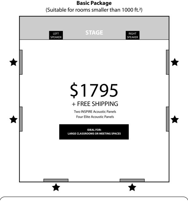
Place 4' x 4' acoustic panels at each of the first reflection points in the room. This will improve clarity and reduce echo and distortion.
